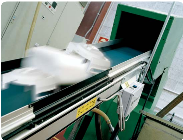
A band conveyor with optional sound trap results in quieter granulation.
