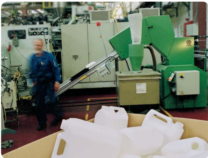
Typical granulator configuration used for blow-moulding applications.
