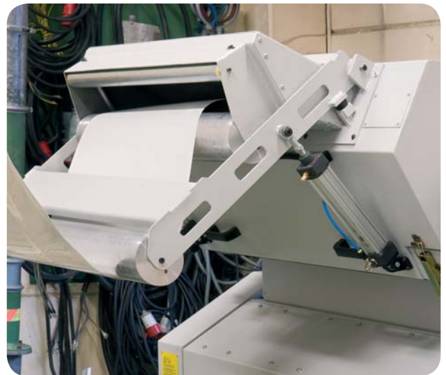
In-line granulator for film granulation. Optional, pneumatic loop control arm for synchronizing film feeding speed with the line speed.
