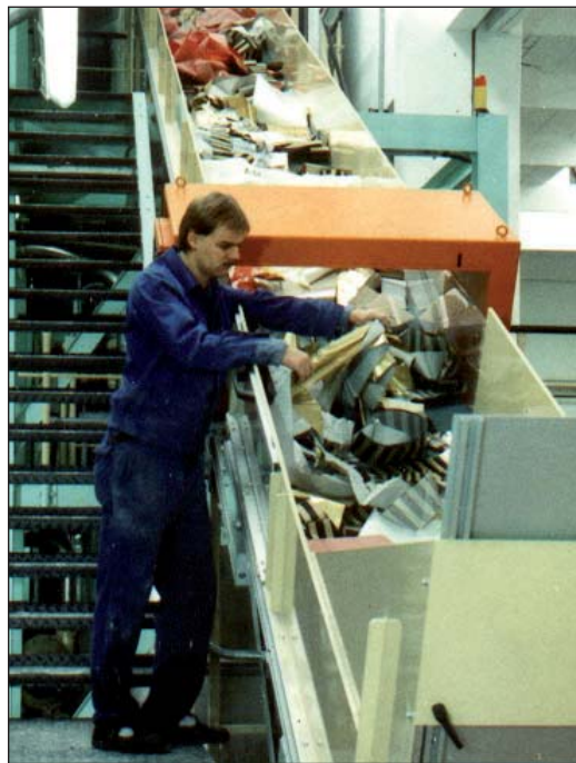
DLS tunnel metal detector inspecting for metal residues
