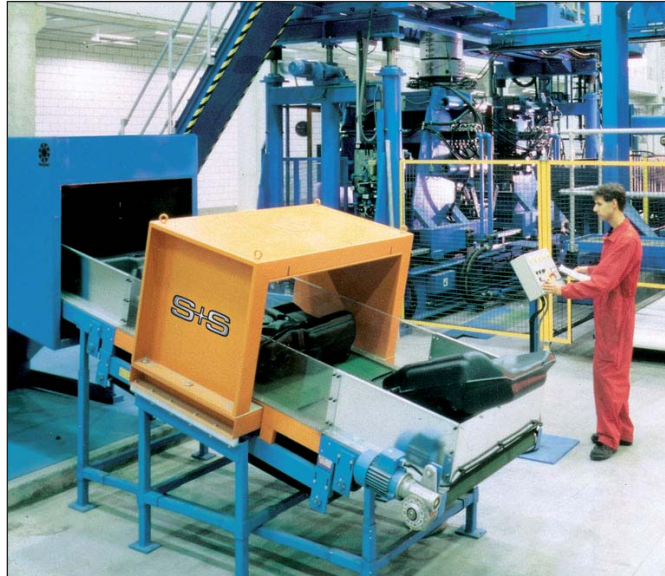
DLS tunnel metal detector inspecting plastic tanks
