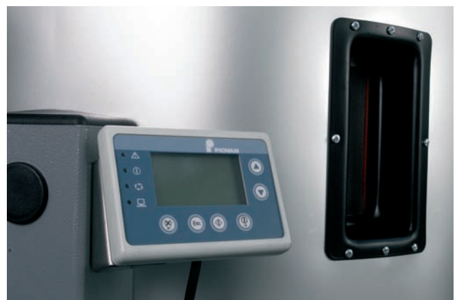
The drying hopper's control
