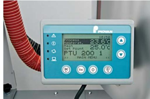
Once the process temperature has been selected, the microprocessor automatically sets the safety temperature within the whole range of functioning temperatures, thus ensuring the maximum operational safety.
