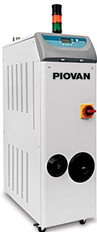
The HR dryers are equipped with two side channel blowers, one dedicated to the process and rotor cooling phases, the other to the regeneration phase. The drying process is independent from the ambient conditions, with consistent Dew Point, with values ranging from -25°C to -50°C.
