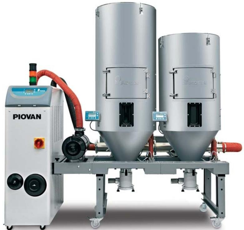
In the **PTU multi-hopper configuration**, the dryer can be connected with 8 drying hoppers maximum, all of which are equipped with a dedicated electronic control. Moreover every single drying hopper is supplied with an independent heating chamber for drying different materials at different temperatures. The PTU system can also include an **integrated vacuum unit**, for loading the material into the drying hoppers of the trolley.
